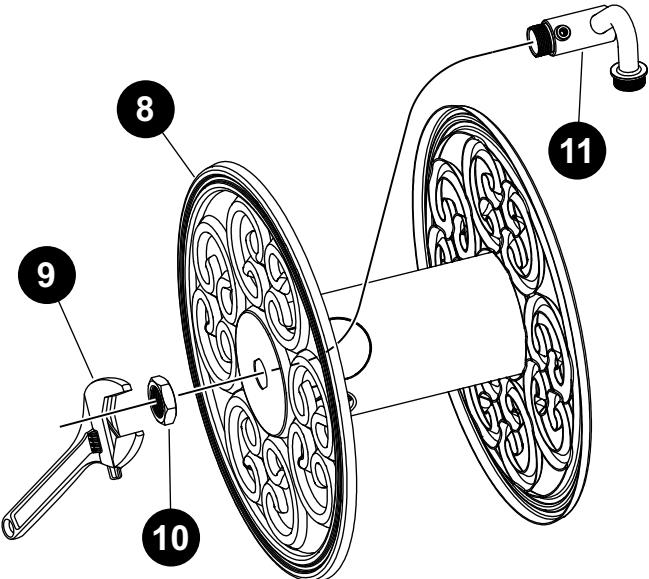
**5** Assemble the elbow (11) and the nut (10) in the hose reel (8). Use an adjustable wrench (9) to tighten the nut.
