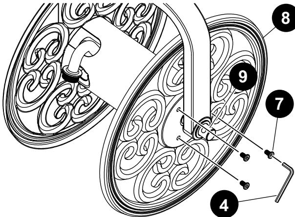
**7** Assemble the swivel (6) and screw (5). Using a hex wrench (4), tighten screw.
