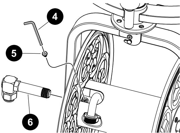
**8** Assemble the crank handle (3) and screw (2). Using a hex wrench (4) tighten screw as shown below.
