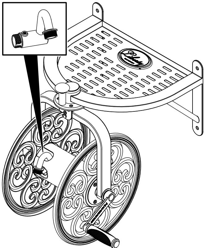
**1** Using a hex wrench (1), remove the screw (2), and remove the crank handle (3).
