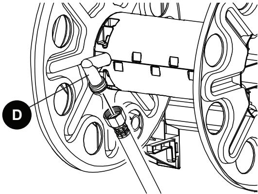
**NOTE:** Check for leaks prior to mounting.
