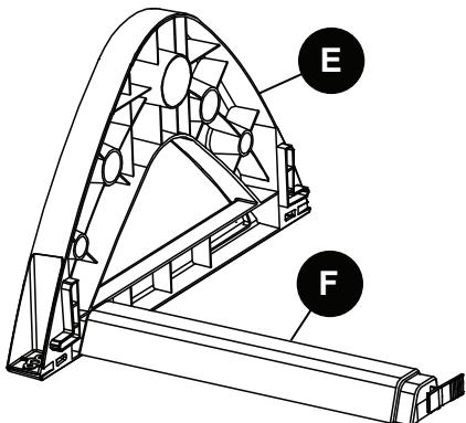
**NOTE:** To disassemble a lower frame bar from a side frame, use a flat head screwdriver to press the lock tab and slide the frame bar out of the snap.
