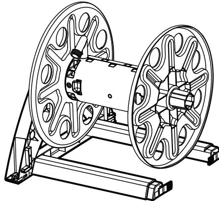
**10.** Install the side frame (E) onto the right reel side (C) and the lower and upper frame bars (F) and (G) as shown.
