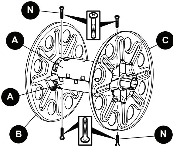
**8.** Ensure the cross brace screws (N) secure both cross braces (A) into the left and right reel sides (B) and (C). See figure below for reference.
