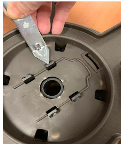
3. Remove the old elbow from the center of the spool.
