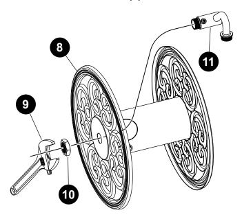
Assemble crank shaft (9), hose reel (8), and screws (7) as shown in the figure below. Tighten the screws with hex wrench (4).
