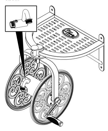
Using a hex wrench (1), remove the screw (2), and remove the crank handle (3).
