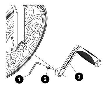
Using a hex wrench (4), remove the screw (5) and remove the swivel (6).
