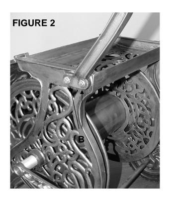
Align the U-handle with the holes in the frame. Take the U-handle bolts (B) and tighten them securely.
