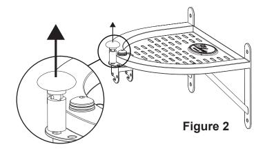
2. Pull up on Locking Pin until Yoke moves freely. **See Figure 2.**
