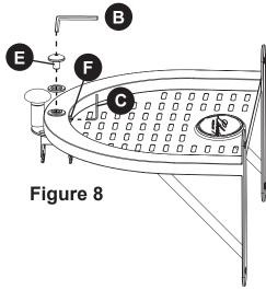
9. Replace Spool onto Yoke. Slide Allen Bolts into holes. Use supplied 4 mm Allen Wrench (C) to hold Allen Bolts in place while using supplied Wrench (D) to tighten Lock Nuts.
