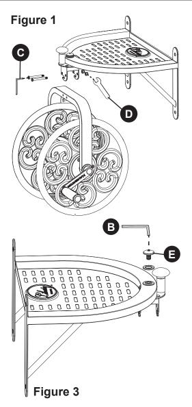
1. First, remove Spool from Yoke by using supplied 4 mm Allen Wrench (C) to hold Allen Bolts in place while using supplied Wrench (D) to remove Lock Nuts. Remove Allen Bolts from holes. To remove Spool from Yoke, lift the Spool upward, then guide it out of small slot on Yoke. Set Spool on ground. See Figure 1.
