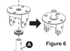
7. Align hole in Replacement Pin (A) with hole in Base Shelf. Insert Small Allen Screw (F) into Base Shelf hole, as shown, and turn with 4 mm Allen Wrench (C) until it catches the Replacement Pin hole.
